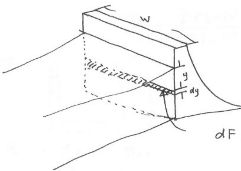
$$\begin{aligned} dF \text{ (at shaded area)} &= p_r \cdot dA \\ &= \rho g y \cdot w \cdot dy \\ &= \rho g w \cdot y \cdot dy \end{aligned}$$
