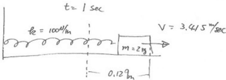
$$\begin{aligned} x &= A \cos(\omega t + \phi) \\ \dot{x} &= -A\omega \sin(\omega t + \phi) \\ \ddot{x} &= -A\omega^2 \cos(\omega t + \phi) \end{aligned} \quad \left. \begin{array}{l} \\ \\ \end{array} \right\} t = 1 \text{ sec} \Rightarrow \left. \begin{array}{l} x = A \cos(\omega t + \phi) = 0.129 \text{ m} \\ \dot{x} = -A\omega \sin(\omega t + \phi) = 3.415 \text{ m/sec} \\ \ddot{x} = -A\omega^2 \cos(\omega t + \phi) \end{array} \right\}$$
