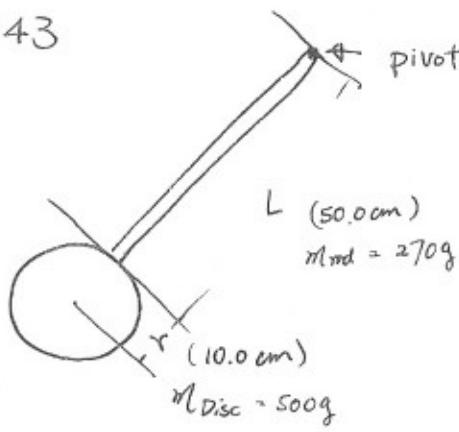
$$(a) I = I_{\text{rod}} + I_{\text{disc}}$$
