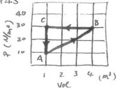
As you can see  $\overline{AB}$  is the time when the positive work is done to the system, and  $\overline{BC}$  is when the system is doing the work (Energy is going out). No work is done during  $\overline{CA}$ . Also notice that the system is releasing more energy to outside ( $\overline{BC}$  phase) than taking ( $\overline{AB}$  phase). The net change is the area of the triangle ABC.
