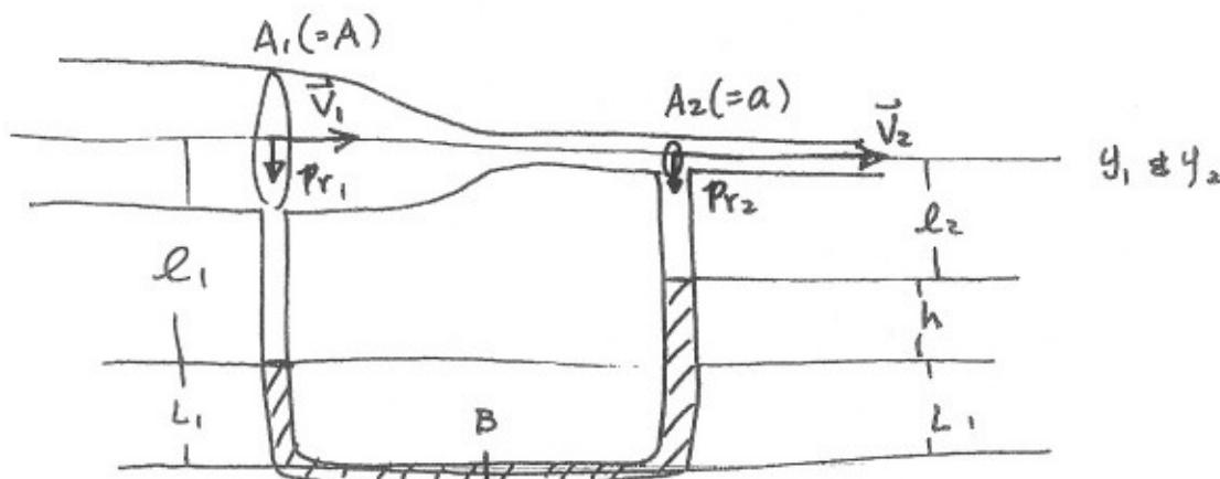
$$Pr_1 + \rho g y_1 + \frac{1}{2} \rho V_1^2 = Pr_2 + \rho g y_2 + \frac{1}{2} \rho V_2^2 \quad (y_1 = y_2)$$
