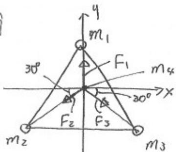
This setting is exactly the same as the Lab #1, first set up (3 forces separated by  $120^\circ$  from each). So,  $\sum \vec{F} = 0$ , and  $|F_1| = |F_2| = |F_3|$  is what we expect to see.
