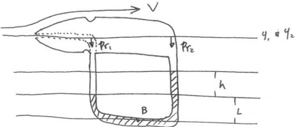
$$P_{r1} + \rho_{air} g q_1 + \frac{1}{2} \rho_{air} V_1^2 = P_{r2} + \rho_{air} g q_2 + \frac{1}{2} \rho_{air} V_2^2 \quad (q_1 = q_2)$$
