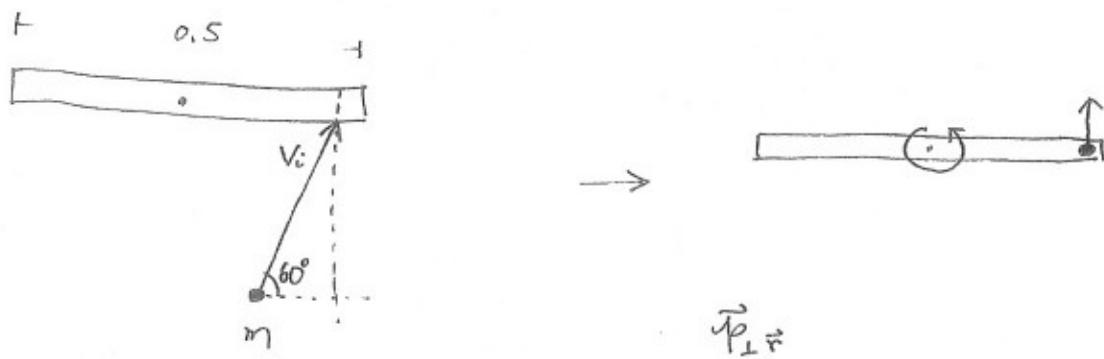
$$\vec{\ell}_i = \vec{r} \times \vec{p} = 0.25 \cdot \overbrace{m_b V_i \sin 60^\circ}^{m_b V_i \sin 60^\circ}$$
