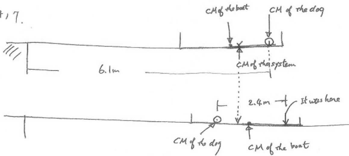
CM of the system will not move. Let  $x$  be the distance that CM of the boat moved (away from the shore). Then,  $(2.4 - x)$  is the distance that the dog moved closer to the shore.
