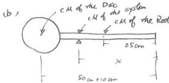
$$X (M_{\text{disc}} + M_{\text{rod}}) = 60 \text{ cm} (M_{\text{disc}}) + 25 \text{ cm} (M_{\text{rod}})$$
