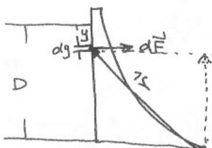
$$\begin{aligned} d\vec{T} - \vec{r} \times d\vec{F} &= (D-y) p_r \cdot dA \\ &= (D-y) (\rho g y) \cdot w \cdot dy \\ &= \rho g w (Dy - y^2) dy \\ \therefore T &= \int d\vec{T} = \int_0^D \rho g w (Dy - y^2) dy \\ &= \rho g w \left( \frac{1}{2} Dy^2 - \frac{1}{3} y^3 \right) \Big|_0^D \\ &= \rho g w \left( \frac{1}{2} D^3 - \frac{1}{3} D^3 \right) \\ &= \underline{\underline{\frac{1}{6} \rho g w D^3}} \end{aligned}$$
