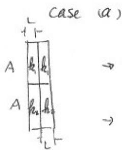
$$\left. \begin{array}{l} P_1 = k_1 \frac{A(T_H - T_C)}{2L} \\ P_2 = k_2 \frac{A(T_H - T_C)}{2L} \end{array} \right\} P_T = P_1 + P_2 = (k_1 + k_2) \frac{A(T_H - T_C)}{2L} \quad \text{--- (1)}$$
